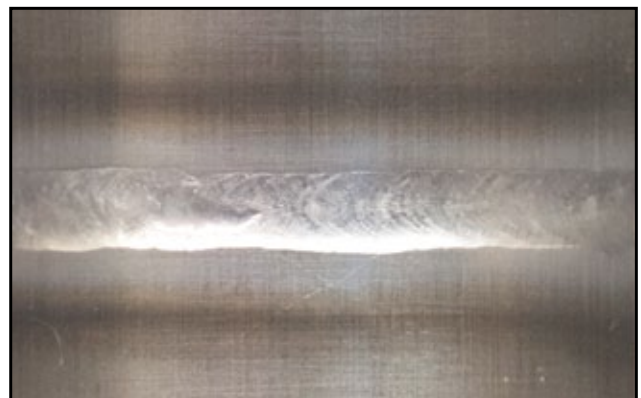
Acceptable weld made in AL-6XN mechanically polished tubing
