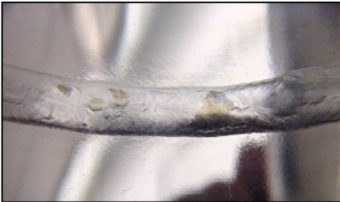
Acceptable weld made in AL-6XN electropolished tubing
